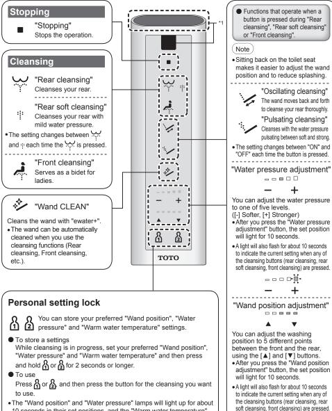
10 seconds in their set positions, and the "Warm water temperature" display switches.
