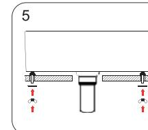
After aligning with the mounting holes place the lavatory on the washstand and attach the lavatory as shown.
