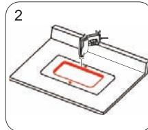
Drill the cutout around mounting holes, cut out the holes for the drain and the water tap.
