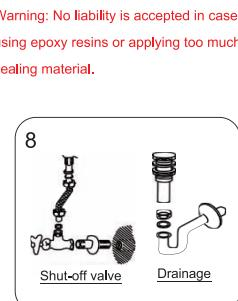
After the sealing material has hardened, the washstand can be installed as intended.
