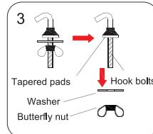
Remove washer and butterfly nut from hook bolts on the product, leaving only tapered pads on the hook bolts.
