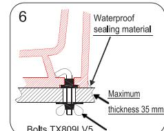
The washstand must be no more than 35 mm thick.
