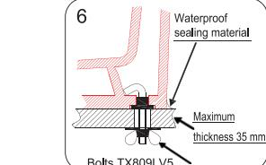
**Warning:** No liability is accepted in case of using epoxy resins or applying too much sealing material.
