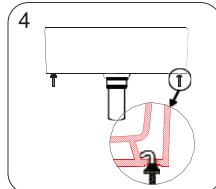
The hook bolts are placed on both sides through the mounting holes at the underside of the lavatory.
