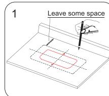
Position the template according to the installation place and mark the cutout for the lavatory.
