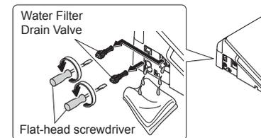
**5** When water draining is completed, reinstall the two water filter drain valves.
