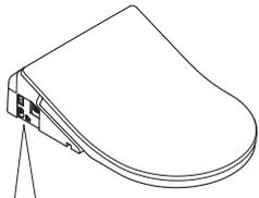
Water filter drain valve
