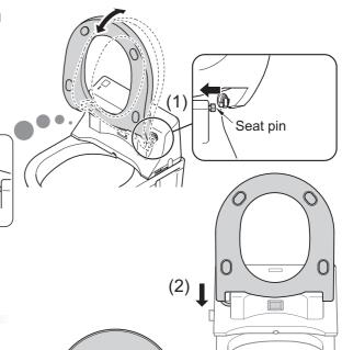
With the lever at the bottom left in the outwards position, reattach the lid as shown in the illustration.
