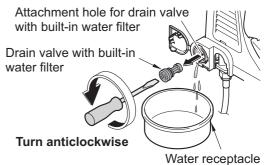
(4) Lift the water supply hose to drain the water out of it.
