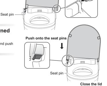
Replacing the seat pins
