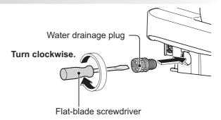
Use a flat-blade screwdriver to tighten it thoroughly.
