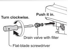
Use a flat-blade screwdriver to tighten it thoroughly.
