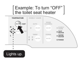
Press the temperature adjustment button repeatedly until the temperature adjustment lamp goes out.
