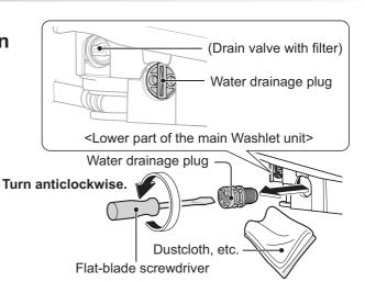
Use a flat-blade screwdriver to loosen the water drainage plug.
