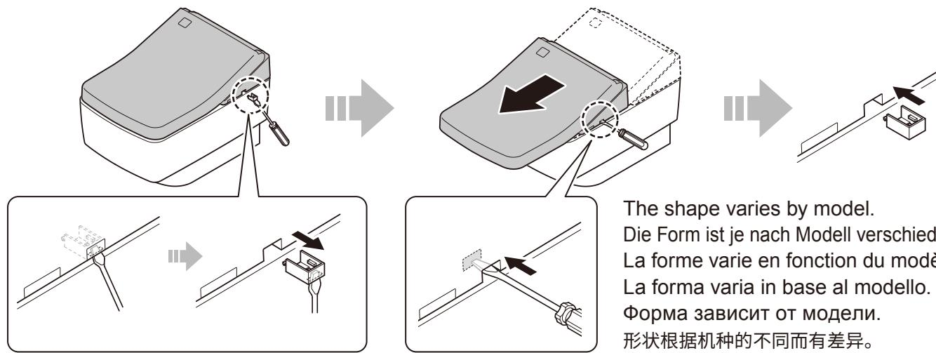
\*Confirm that no power is applied and no water is inside the product, align the position and install it again.
